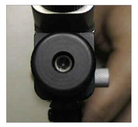
Turning the screw clockwise on the mainspring tension screw increases the mainspring tension and increases the velocity and the recock gas expulsion. Turning the mainspring tension screw counterclockwise decreases tension on the mainspring and decreases the inertia gained by the the hammer. The hammer strikes the poppet valve with less pressure, which decreases the gas flow, which in turn decreases the velocity and / or the recocking action.
