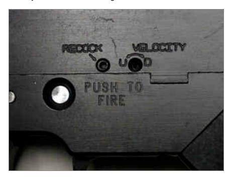
Turning the VELOCITY or RECOCK adjustment screws in the clockwise direction restricts the gas flow to either the velocity or recock. Turning the screw counterclockwise increases gas flow, thus increasing the gas used to propel the paintball or the recocking action. These adjustment screws labeled VELOCITY and RECOCK are used to balance the use of the gas
