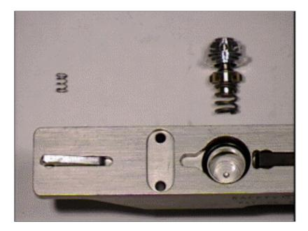
The gun has a leak around the VTS or VATS adapter seam. Reason: The seal between the VTS or VATS adapter and the lower receiver is bad.
